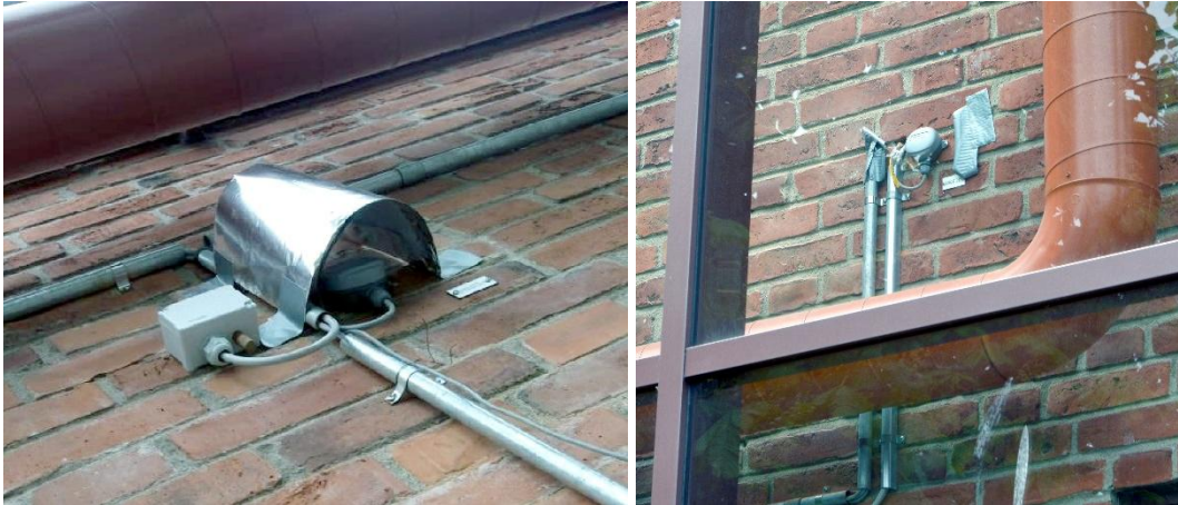
Figure 26. Temperature sensor shielded with aluminum foil (left) [189]. The aluminum foil from some sensors was removed for the measurements (right).
