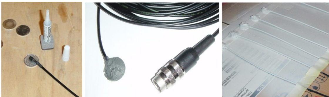
Figure 15. Photos of the assembly of the surface temperature sensor [19]
